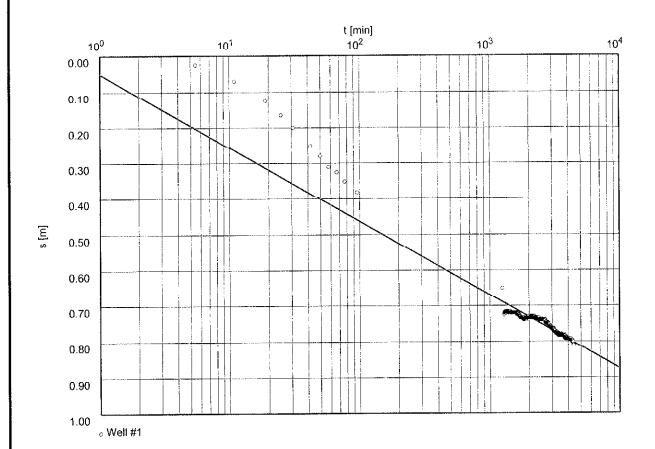
Transmissivity [m²/min]: 1.79 x 10<sup>-1</sup>
