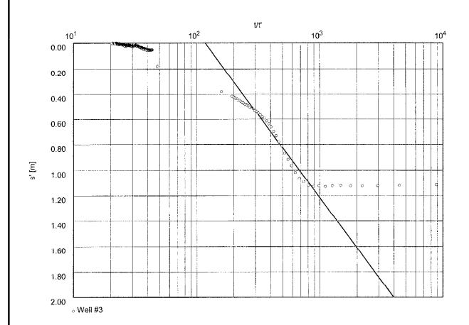
Transmissivity [m²/min]:  $2.72 \times 10^{-2}$
