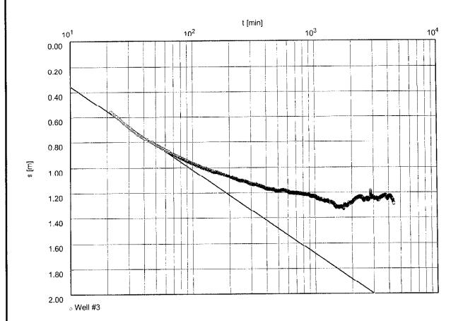
Transmissivity [m²/min]: 5.37 x 10<sup>-2</sup>
