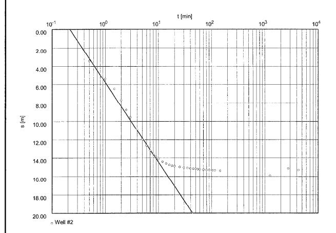
Transmissivity [m²/min]:  $4.11 \times 10^{-3}$
