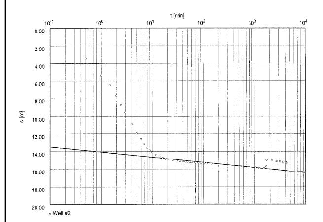
Transmissivity [m²/min]: 6.09 x 10<sup>-2</sup>
