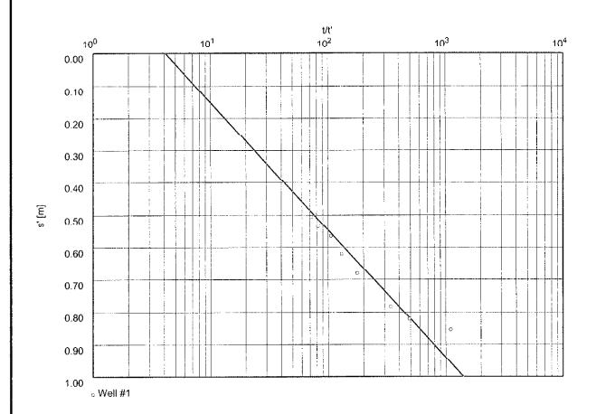
Transmissivity [m²/min]:  $9.39 \times 10^{-2}$
