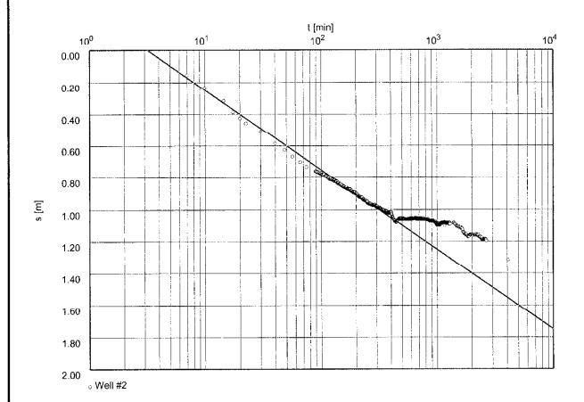
Transmissivity [m²/min]:  $7.39 \times 10^2$
