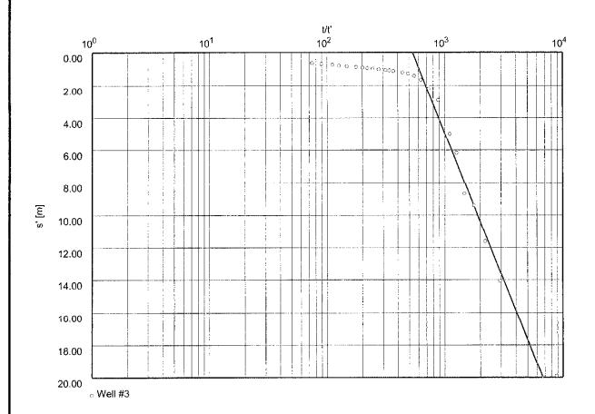
Transmissivity [m²/min]: 2.03 x 10<sup>-3</sup>
