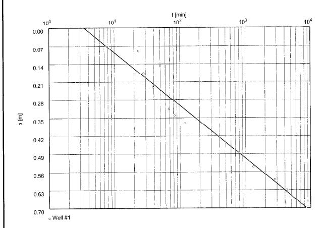
Transmissivity [m²/min]: 1.73 x 10<sup>-1</sup>
