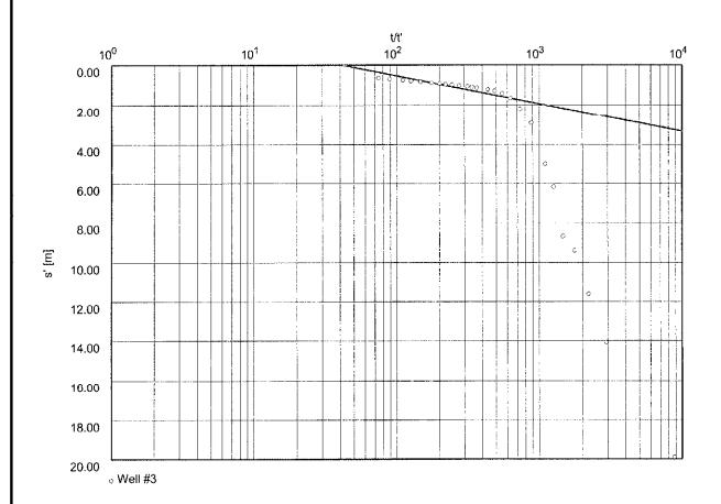
Transmissivity [m²/min]:  $2.64 \times 10^{-2}$
