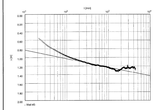
Transmissivity [m²/min]: 1.78 x 10<sup>-1</sup>
