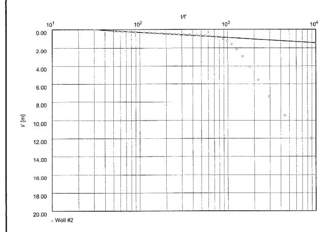
Transmissivity [m²/min]: 6.24 x 10<sup>-2</sup>
