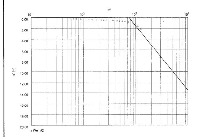
Transmissivity [m²/min]:  $2.97 \times 10^3$
