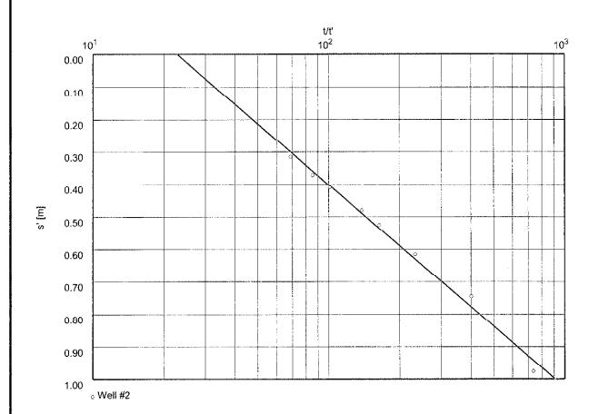
Transmissivity [m²/min]: 5.93 x 10<sup>-2</sup>
