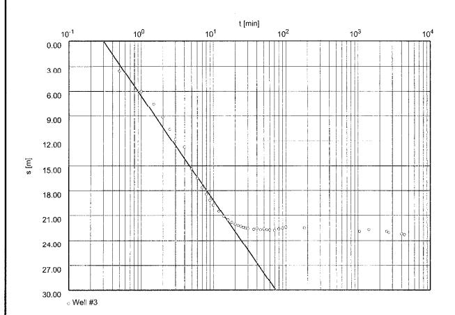
Transmissivity [m²/min]: 2.94 x 10<sup>-3</sup>
