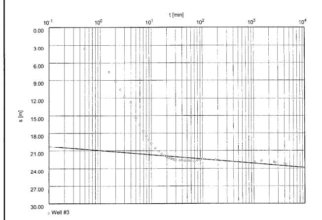
Transmissivity [m $^2$ /min]: 5.18 x 10 $^2$
