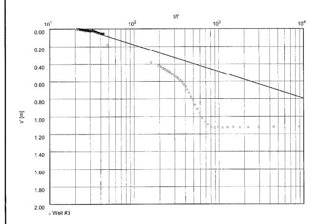
Transmissivity [m²/min]: 1.17 x 10<sup>-1</sup>
