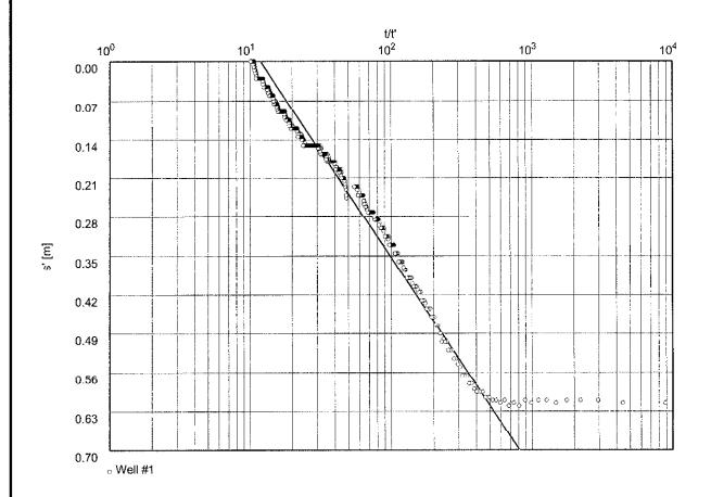
Transmissivity [m²/min]:  $9.34 \times 10^{-2}$
